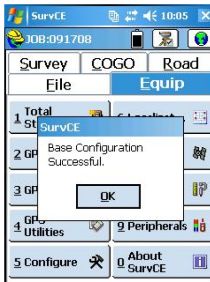
Figure 28: Successful Base Station Configuration
